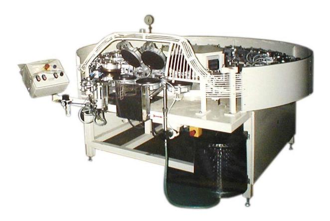
It is the same construction like PK 21 R, 2 X A, but operated by hand. This means that this machine does not come with the manipulator and the reservoir. The machine can be used individually or in not-automatic production lines of the production of the spa-wafers or triangular wafers.
